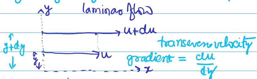
Shear stress & transverse velocity gradient
